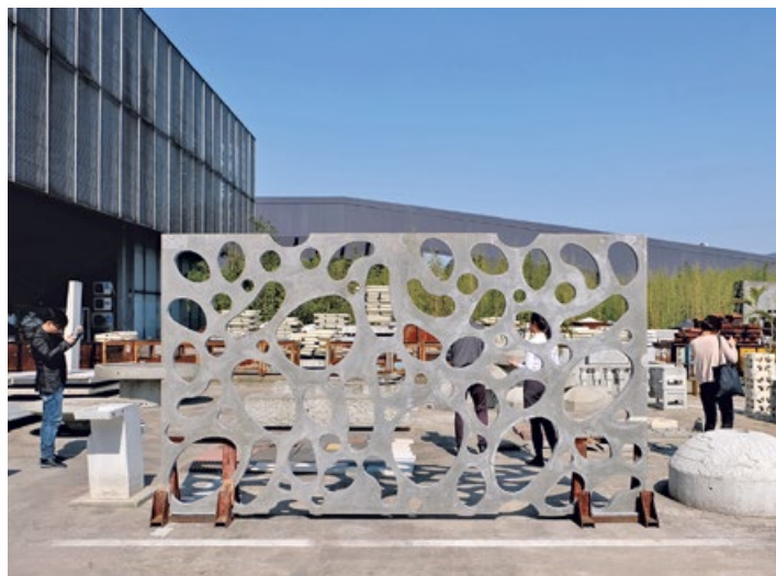
The prototype yard at the Vanke Architecture Research Centre, showing a segmental mock-up of a decorative concrete facade element.
