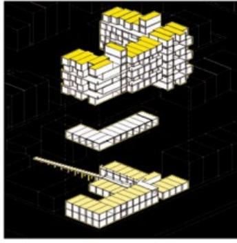
SUPER-STRUCTURE: Interim housing installed on top of a new but permanent base building
