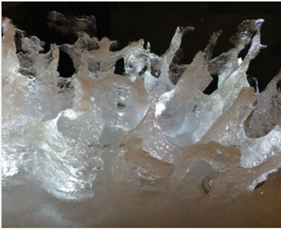
above and opposite: A bespoke ice 3D-printing technique was developed that could be utilised for 3D printing high-resolution porous cavity wall ice constructions.
